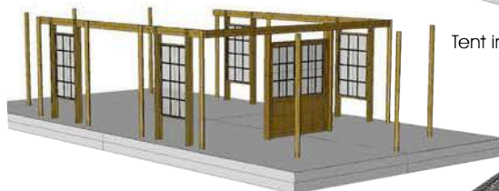
Wood legs with windows and doors installed
