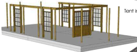
Wood legs with windows and doors installed
